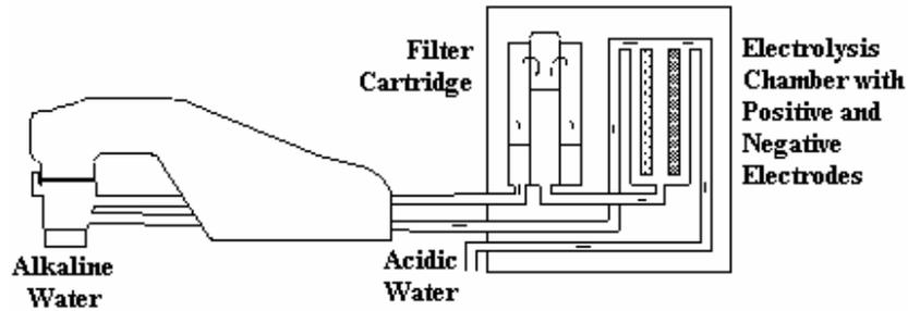
A special attachment re-directs tap water out of the faucet through a plastic hose into the Ionized Water unit. Inside the Ionized Water unit, the water is first filtered through activated charcoal. Next, the filtered water passes into an electrolysis chamber equipped with a platinum-coated titanium electrode where electrolysis takes place.
